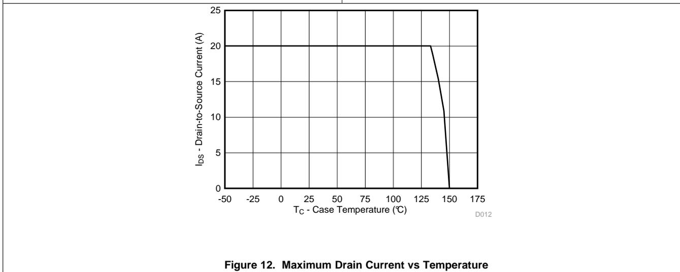
**Figure 12. Maximum Drain Current vs Temperature**
