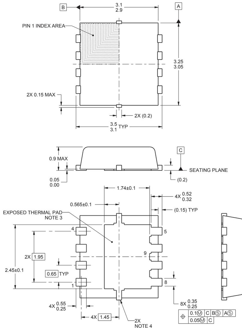
1. All linear dimensions are in millimeters. Any dimensions in parenthesis are for reference only. Dimensioning and tolerancing per ASME Y14.5M.
