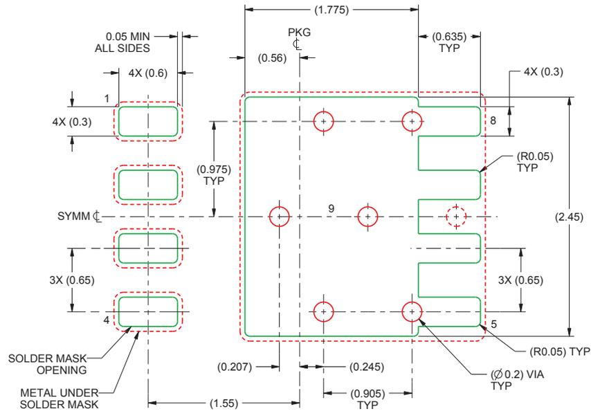
1. This package is designed to be soldered to a thermal pad on the board. For more information, see *QFN/SON PCB Attachment* application report, [SLUA271](#).
