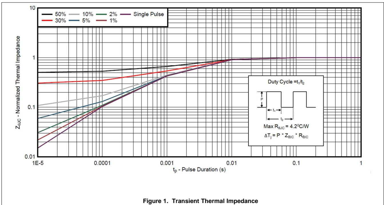
Figure 1. Transient Thermal Impedance
