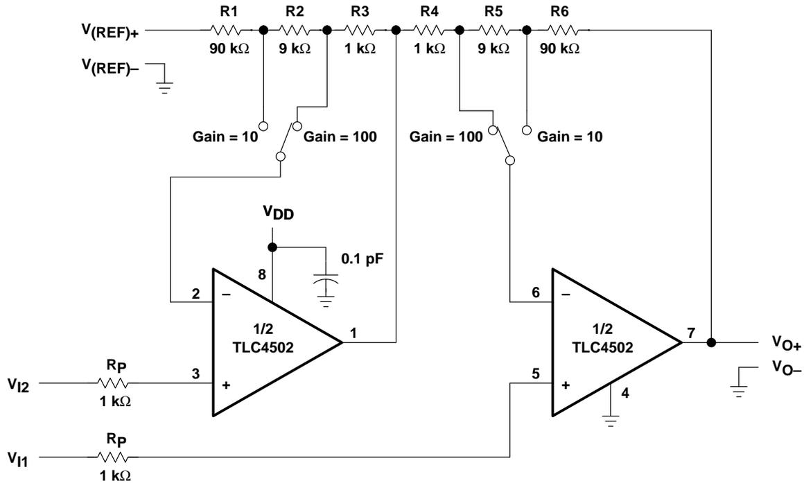
$$\text{(Gain = 10)} \quad V_O = (V_{I1} - V_{I2}) \left( 1 + \frac{R_6}{R_4 + R_5} \right) + V_{(REF)} \quad \text{Where } R_1 = R_6, R_2 = R_5, \text{ and } R_3 = R_4$$
