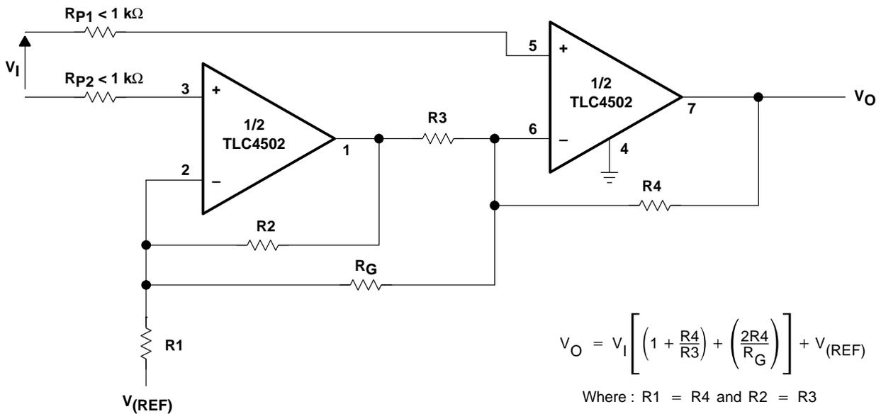
$$V_O = V_I \left[ \left( 1 + \frac{R_4}{R_3} \right) + \left( \frac{2R_4}{R_G} \right) \right] + V_{(REF)}$$
