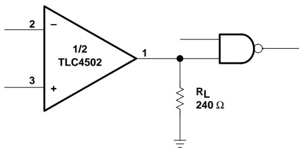
Figure 42. TTL-Driver Circuit
