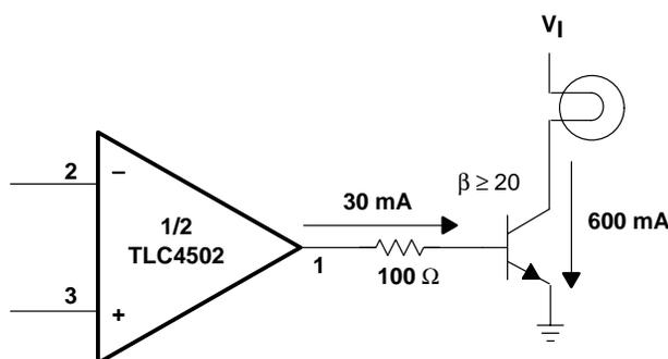
Figure 41. Lamp-Driver Circuit
