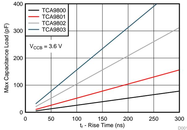
Figure 28. Maximum Load Capacitance vs Rise Time (400-kHz I<sup>2</sup>C, V<sub>CCB</sub> = 3.6 V)
