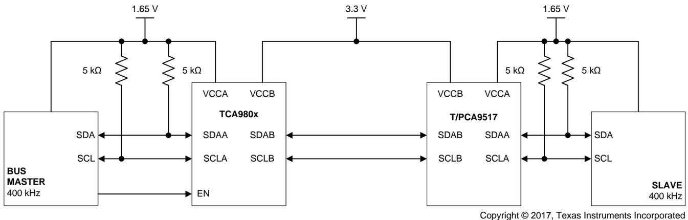
**Figure 17. Incorrect B-Side Static Voltage Offset Buffer Connection**
