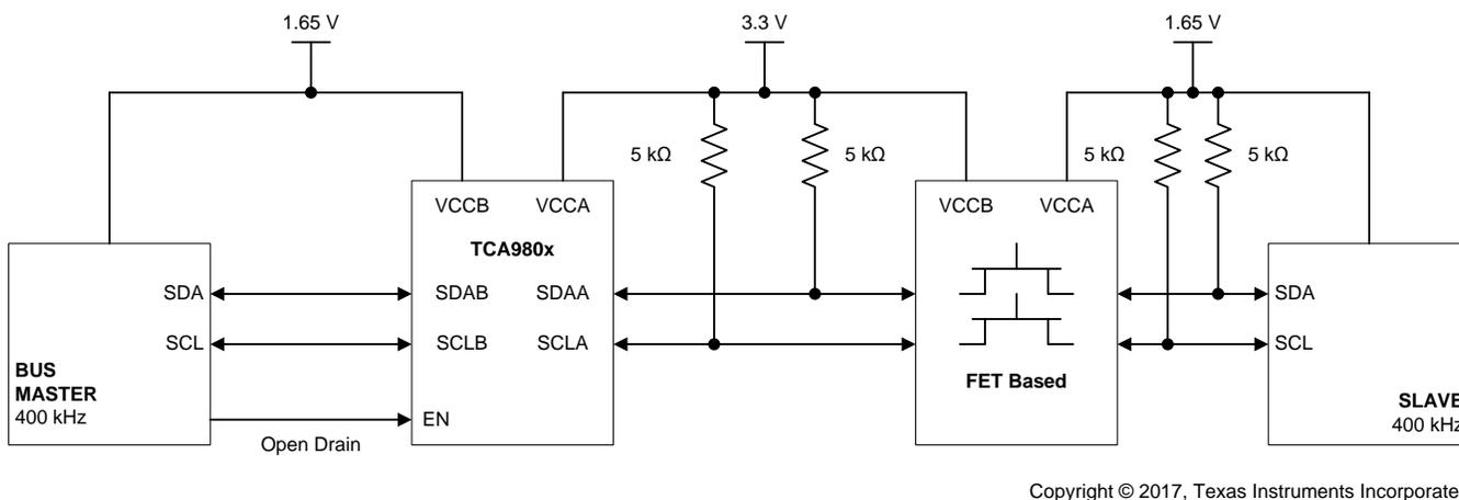
Figure 16. A-Side Pass-Gate Based Translator Use Case
