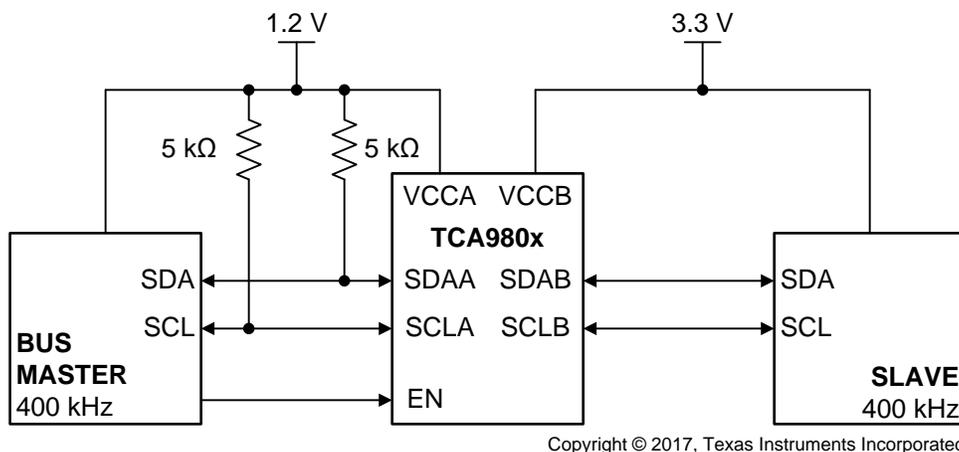
**Figure 19. Typical Level-Shifting Application Example (Master on A-side)**
