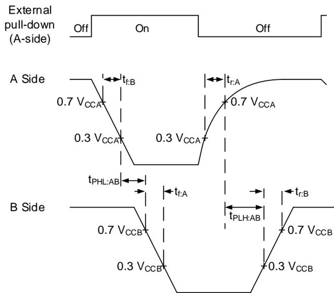
Figure 9. Propagation Delay and Transition Times for A-Side to B-Side
