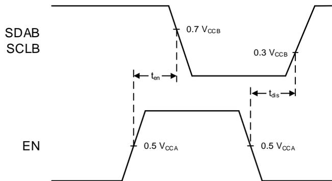
1)  $V_{CCA}$  is powered, SDA/SCLA are connected to GND
