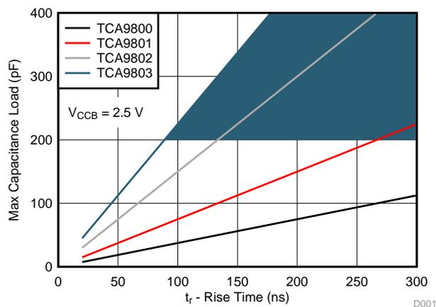
**Figure 30. Selection Guide Based On Example Design Requirements**
