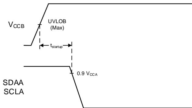
1)  $V_{CCA}$  is powered, SDAB/SCLB are connected to GND
