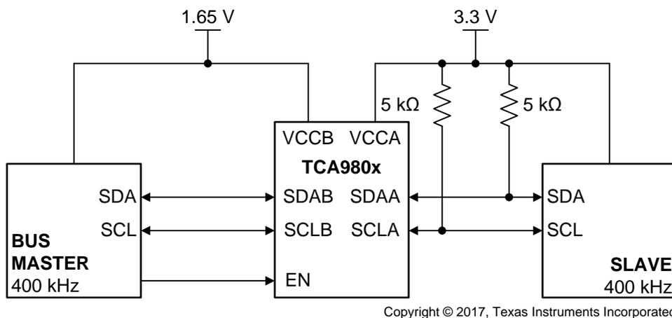
**Figure 20. Typical Level-Shifting Application Example (Master on B-side)**
