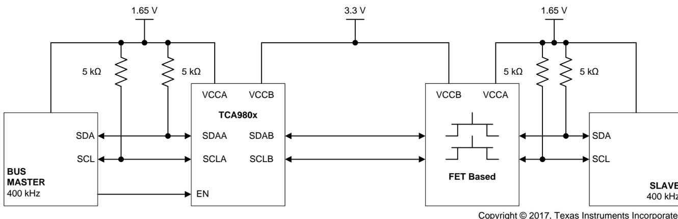
Figure 15. Incorrect B-Side Pass-Gate Based Translator Use Case
