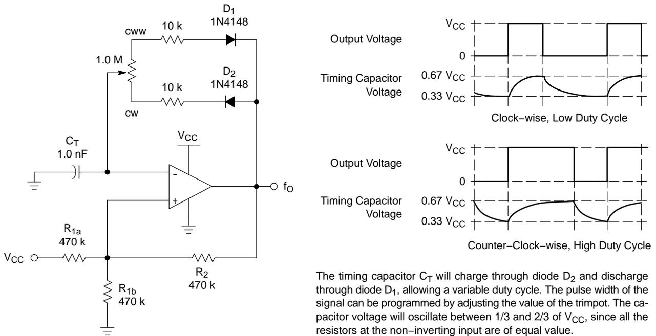
Figure 35. Variable Duty Cycle Pulse Generator
