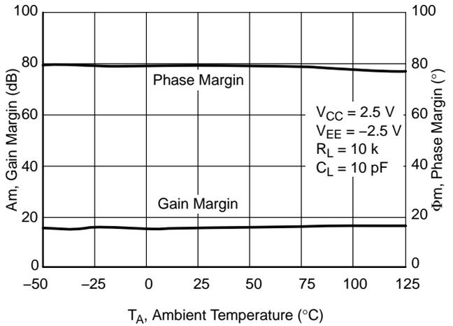
Figure 21. Gain and Phase Margin vs. Temperature
