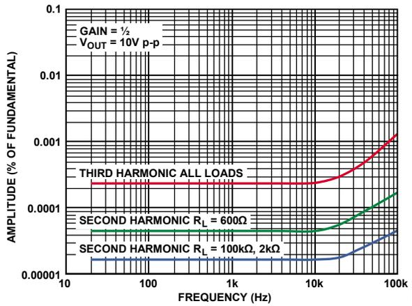
Figure 36. Harmonic Distortion Products vs. Frequency, G = 1/2
