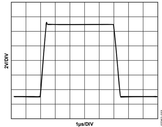
Figure 28. Large-Signal Pulse Response, Gain = 2
