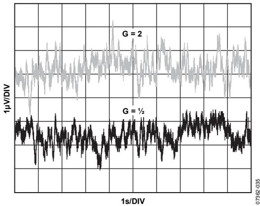
Figure 31. 0.1 Hz to 10 Hz Voltage Noise, RTO
