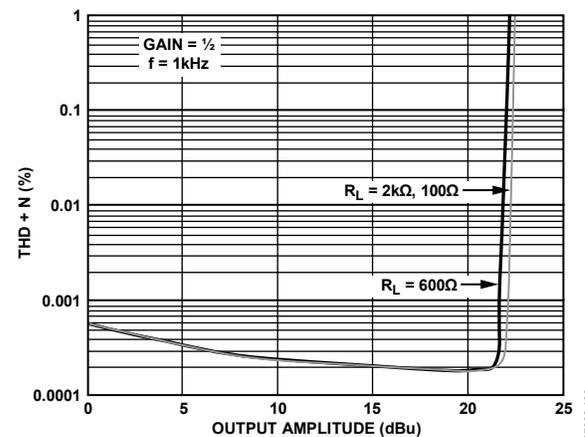
Figure 34. THD + N vs. Output Amplitude, G = 1/2
