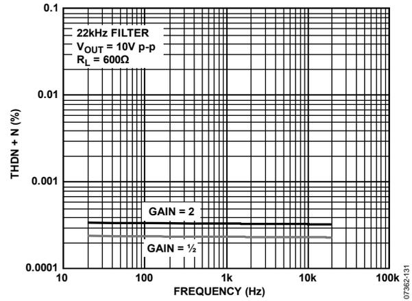
Figure 32. THD + N vs. Frequency, Filter = 22k Hz
