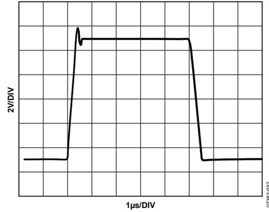
Figure 27. Large-Signal Pulse Response, Gain = 1/2
