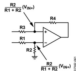
Figure 39. Voltage Division in the Difference Amplifier Configuration
