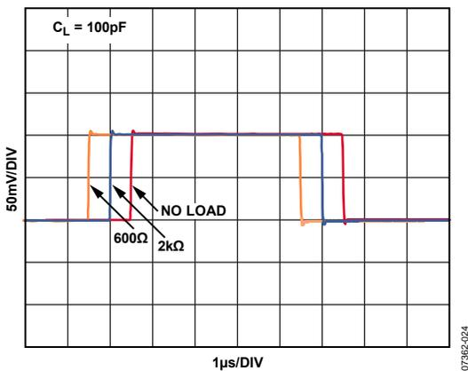
Figure 19. Small-Signal Step Response, Gain = 2
