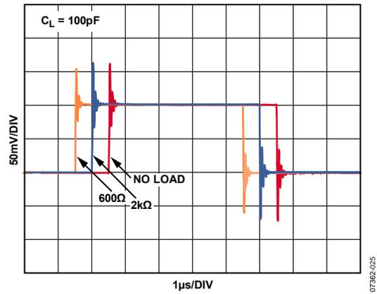
Figure 20. Small-Signal Step Response, Gain =  $\frac{1}{2}$
