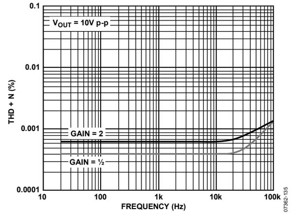
Figure 33. THD + N vs. Frequency, Filter = 120 kHz
