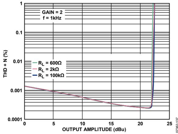
Figure 35. THD + N vs. Output Amplitude, G = 2
