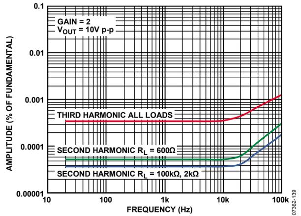
Figure 37. Harmonic Distortion Products vs. Frequency, G = 2
