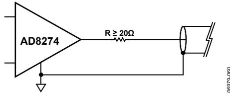
Figure 48. Driving Cabling
