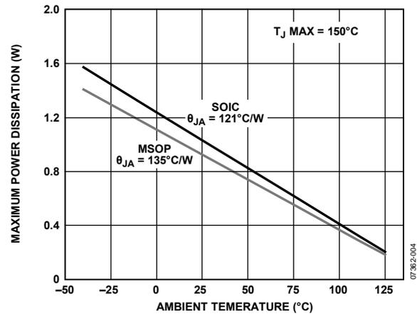
Figure 2. Maximum Power Dissipation vs. Ambient Temperature
