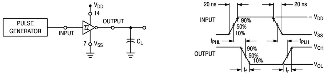
Figure 1. Switching Time Test Circuit and Waveforms
