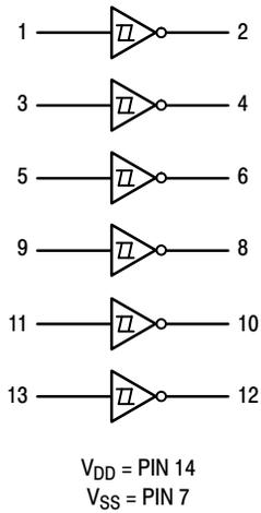
**Figure 1. Logic Diagram**
