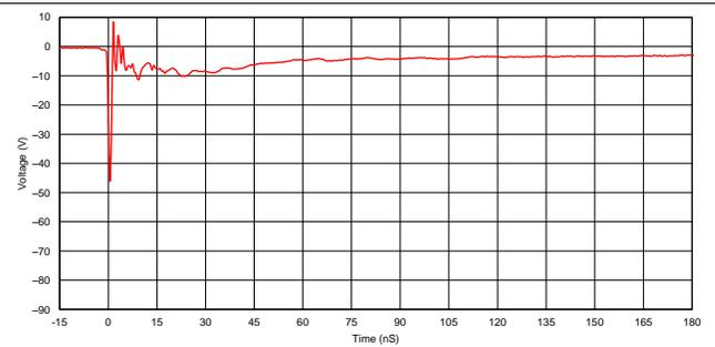
**Figure 2. TPD12S520RMN IEC Clamping Waveforms -8kV Contact**
