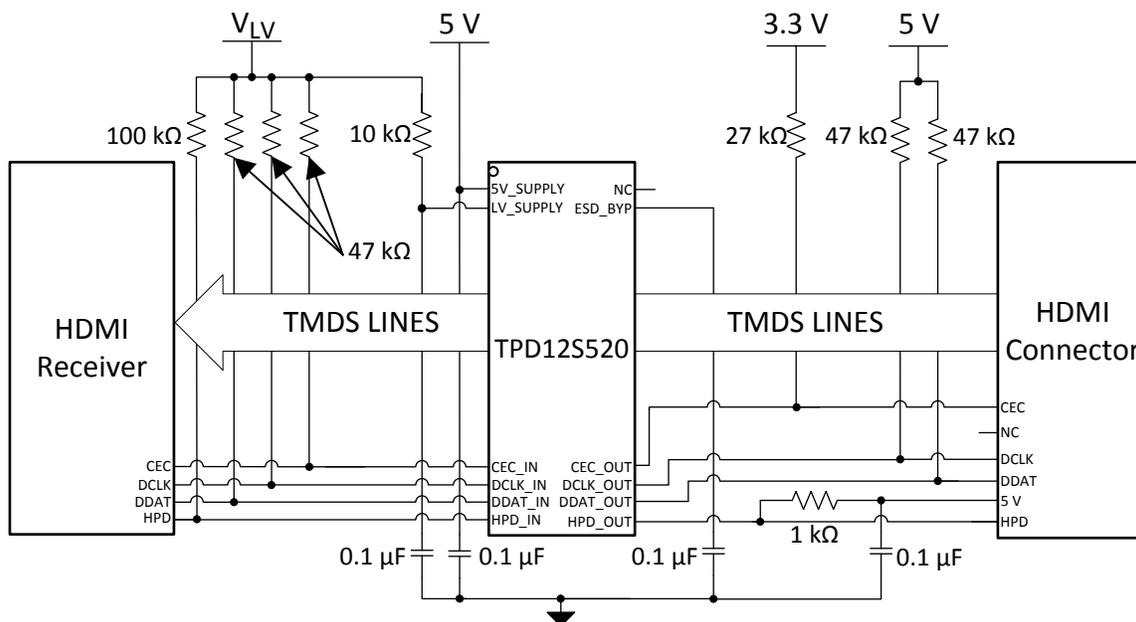
Figure 6. TPD12S520 Configured with an HDMI 1.4 Receiver Port
