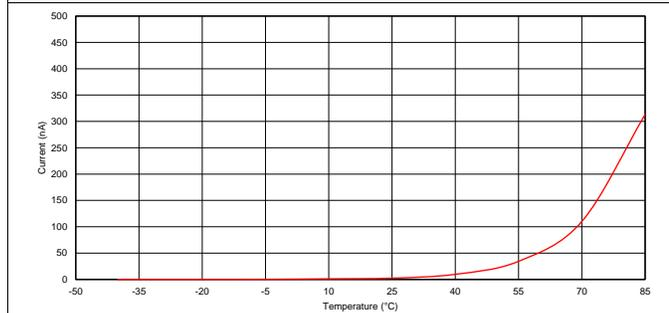
**Figure 3.  $I_{LEAK}$  vs. Temperature  $V_{IN} = 5.0V$**
