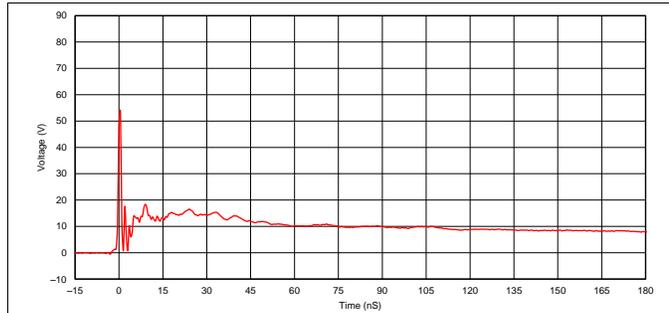
**Figure 1. TPD12S520RMN IEC Clamping Waveforms +8kV Contact**
