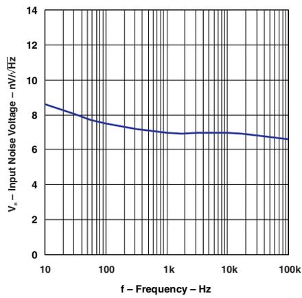
**Figure 13. Input Noise Voltage vs Frequency**
