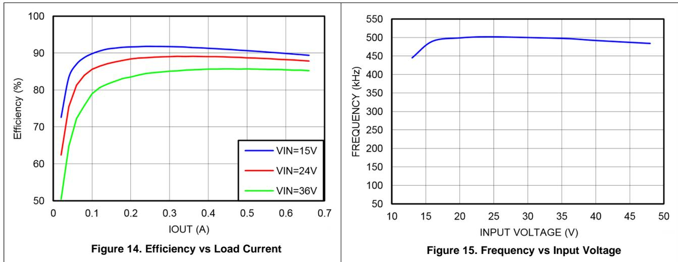
Figure 14. Efficiency vs Load Current
