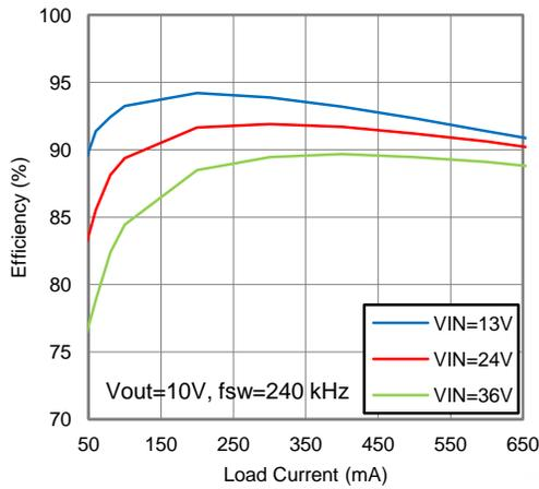
Figure 1. Efficiency at 200 kHz, 10 V
