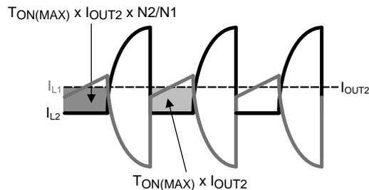
Figure 18. Current Waveforms for  $C_{OUT1}$  Ripple Calculation
