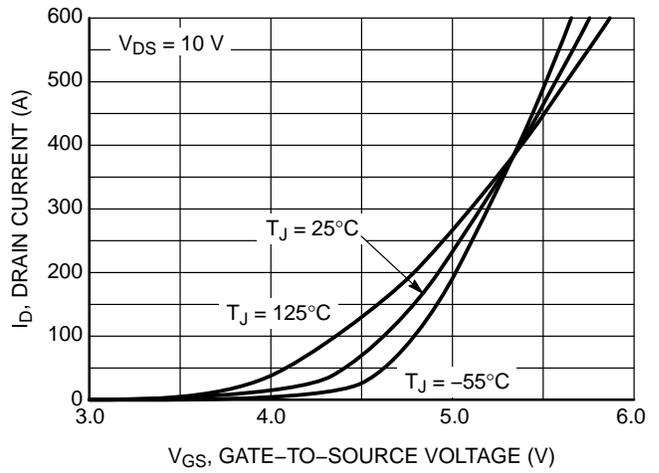
Figure 2. Transfer Characteristics
