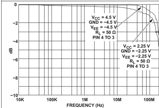
Figure 5. Channel ON Bandwidth (HC and HCT4052)
