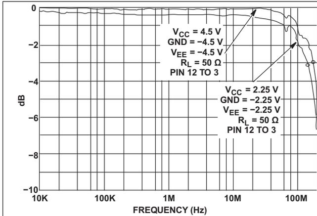
Figure 3. Channel ON Bandwidth (HC and HCT4051)
