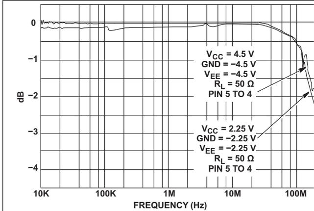
Figure 7. Channel ON Bandwidth (HC and HCT4053)
