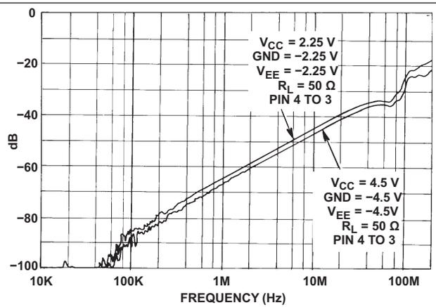
Figure 6. Channel OFF Feedthrough (HC and HCT4052)
