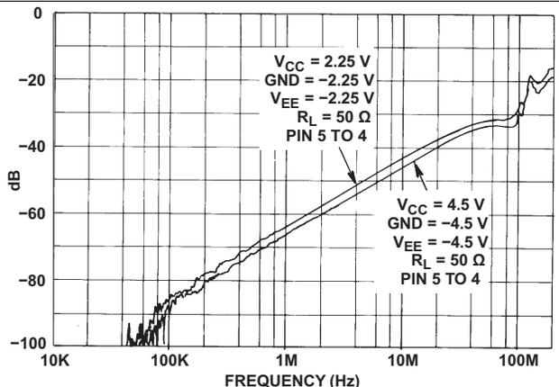
Figure 8. Channel OFF Feedthrough (HC and HCT4053)
