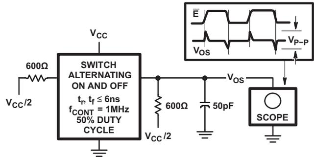
Figure 13. Control to Switch Feedthrough Noise Test Circuit
