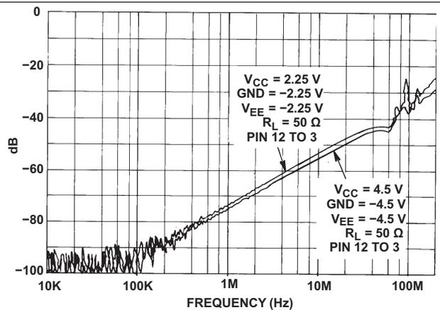
Figure 4. Channel OFF Feedthrough (HC and HCT4051)
