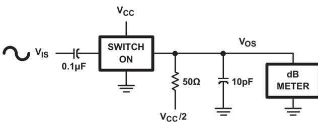
Figure 10. Frequency Response Test Circuit
