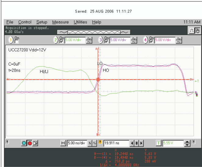
Figure 32. 20-ns Input Pulse Delay Matching
