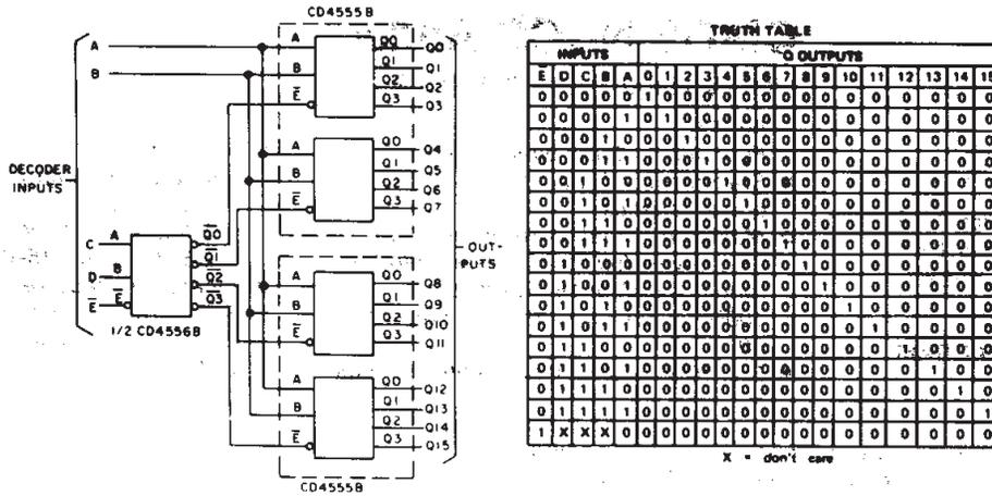
Fig. 21 - 1-of-16 decoder using CD4555B and CD4556B.
