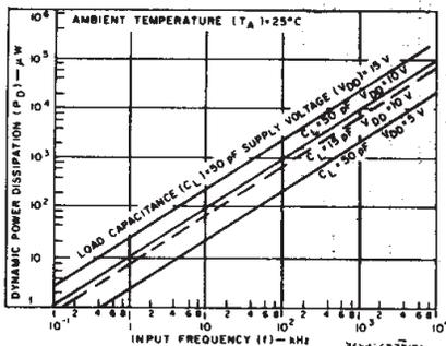
Fig. 11 - Typical dynamic power dissipation vs. frequency.
