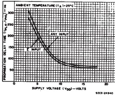
Fig. 9 - Typical propagation delay time vs. supply voltage.
