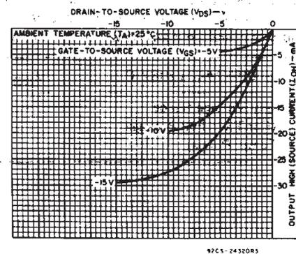
Fig. 3 — Typical output high (source) current characteristics.
