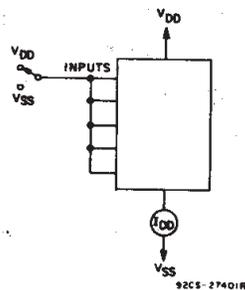
Fig. 12 - Quiescent device current test circuit.
