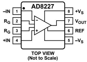
Figure 2. Pin Configuration
