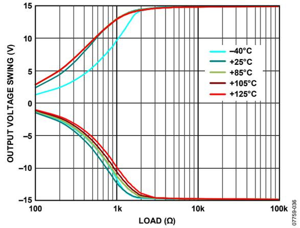
Figure 36. Output Voltage Swing vs. Load Resistance
