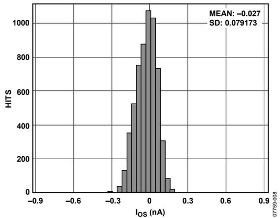
Figure 8. Typical Distribution of Input Offset Current
