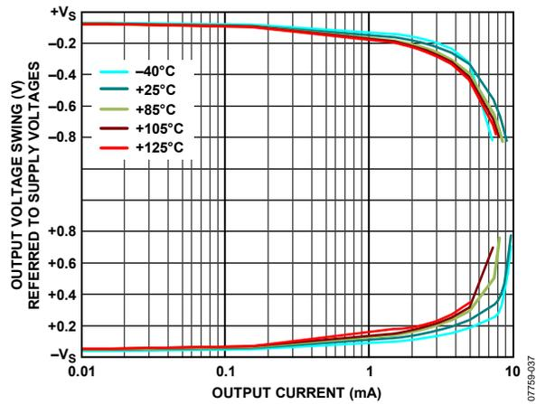
Figure 37. Output Voltage Swing vs. Output Current
