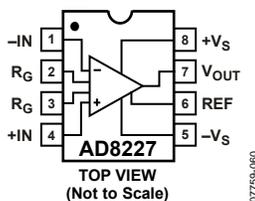
Figure 60. Pinout Diagram
