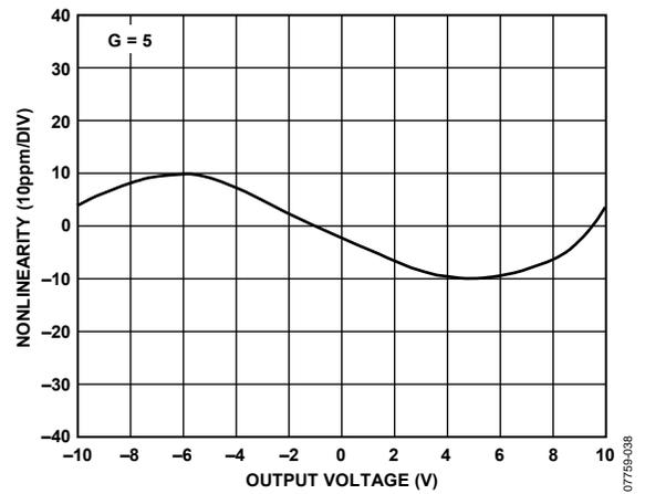
Figure 38. Gain Nonlinearity,  $G = 5$ ,  $R_L \geq 2\text{ k}\Omega$
