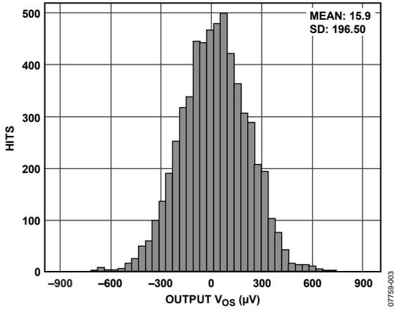
Figure 3. Typical Distribution of Output Offset Voltage
