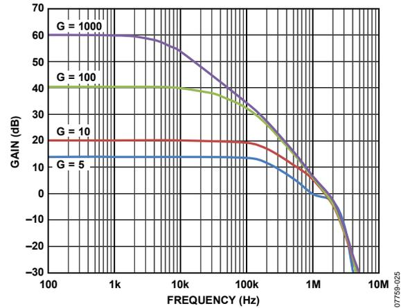
Figure 25. Gain vs. Frequency,  $V_s = \pm 15\text{ V}$
