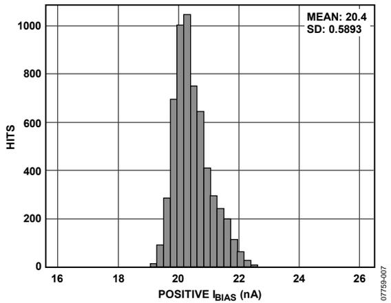
Figure 7. Typical Distribution of Input Bias Current
