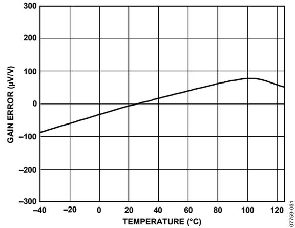
Figure 31. Gain Error vs. Temperature, G = 5
