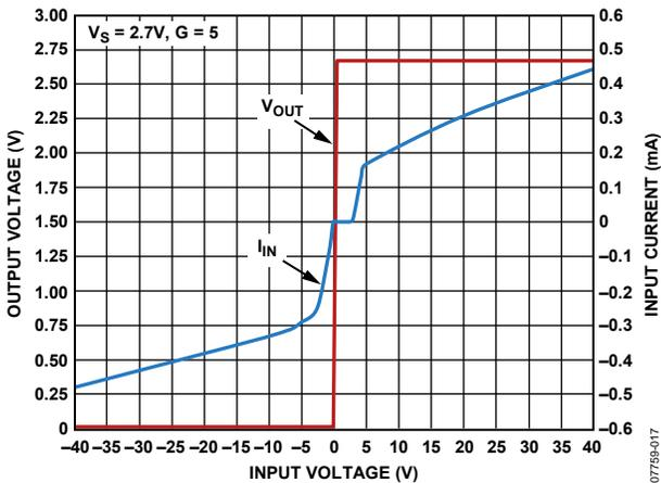
Figure 17. Input Overvoltage Performance,  $G = 5$ ,  $V_S = 2.7\text{ V}$
