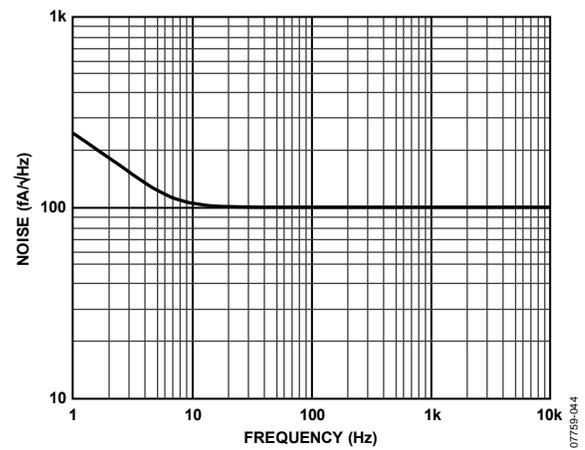
Figure 44. Current Noise Spectral Density vs. Frequency
