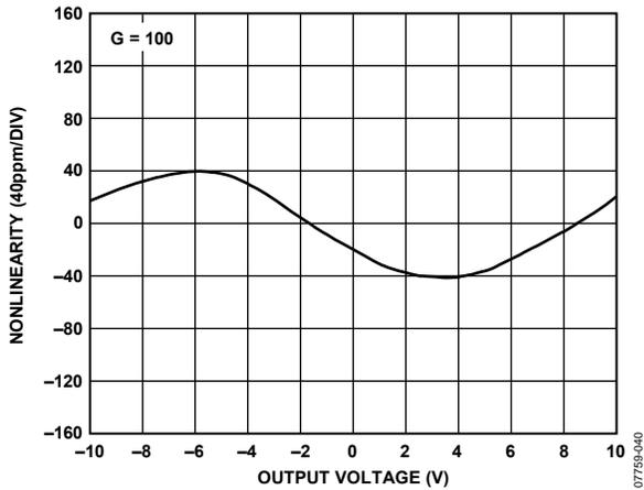
Figure 40. Gain Nonlinearity,  $G = 100$ ,  $R_L \geq 2 \text{ k}\Omega$
