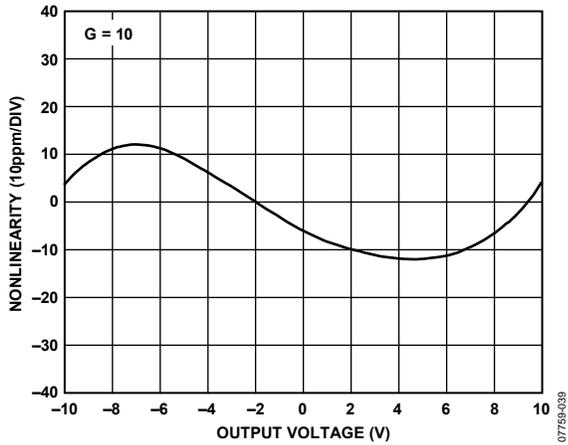
Figure 39. Gain Nonlinearity,  $G = 10$ ,  $R_L \geq 2 \text{ k}\Omega$
