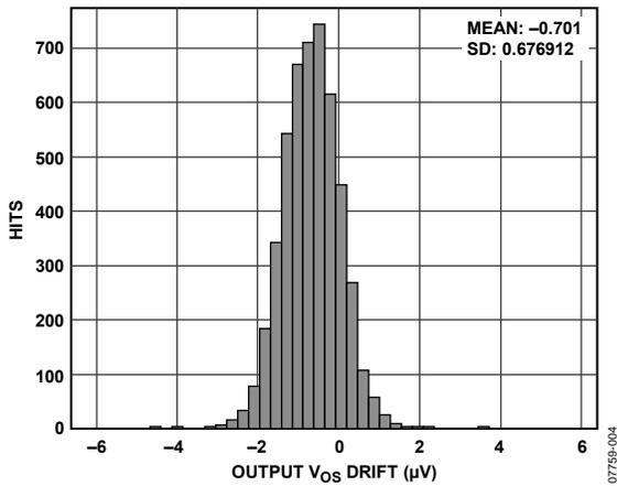
Figure 4. Typical Distribution of Output Offset Voltage Drift
