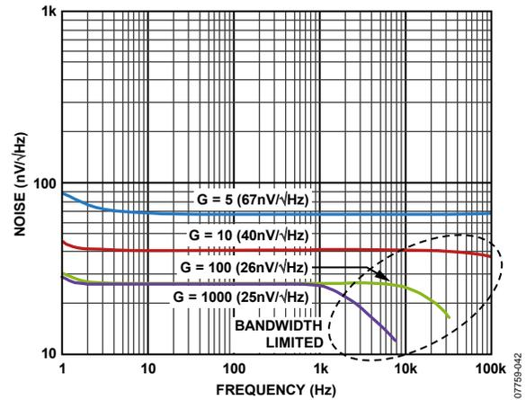
Figure 42. Voltage Noise Spectral Density vs. Frequency
