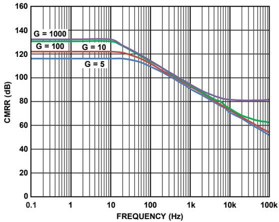
Figure 28. CMRR vs. Frequency, RTI, 1 kΩ Source Imbalance
