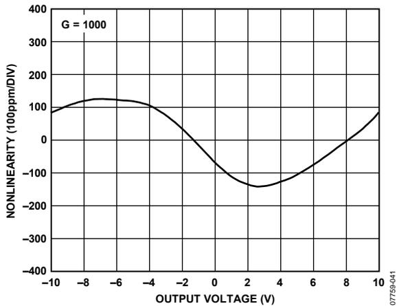
Figure 41. Gain Nonlinearity,  $G = 1000$ ,  $R_L \geq 2 \text{ k}\Omega$
