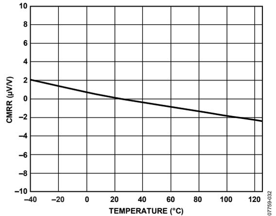
Figure 32. CMRR vs. Temperature, G = 5
