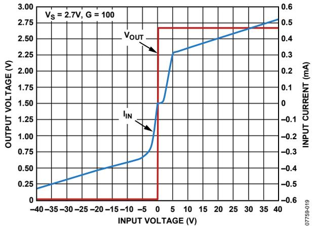
Figure 19. Input Overvoltage Performance,  $G = 100$ ,  $V_S = 2.7\text{ V}$
