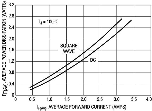
Figure 3. Power Dissipation
