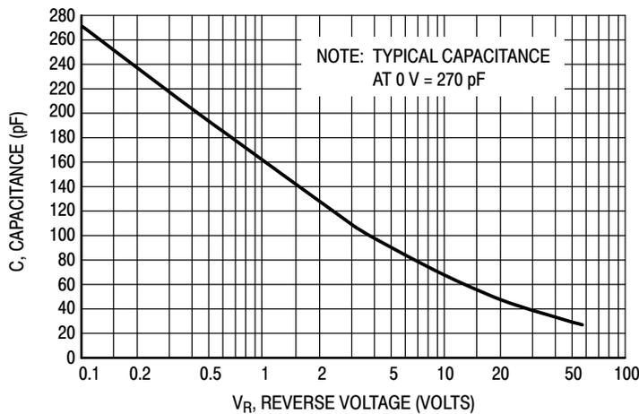
Figure 5. Typical Capacitance
