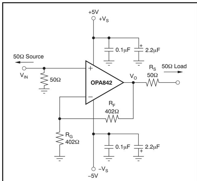
**Figure 37. Gain of +2, High-Frequency Application and Characterization Circuit**
