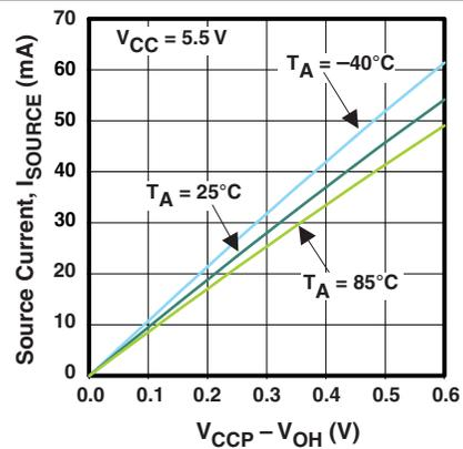
Figure 16. I/O Source Current vs Output High Voltage
