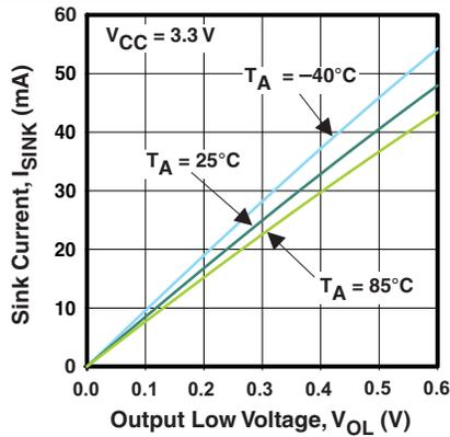
Figure 7. I/O Sink Current vs Output Low Voltage
