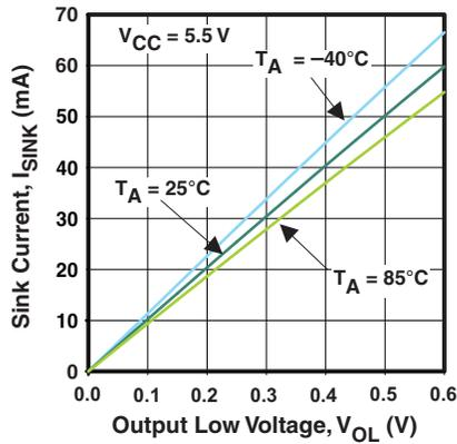
Figure 9. I/O Sink Current vs Output Low Voltage
