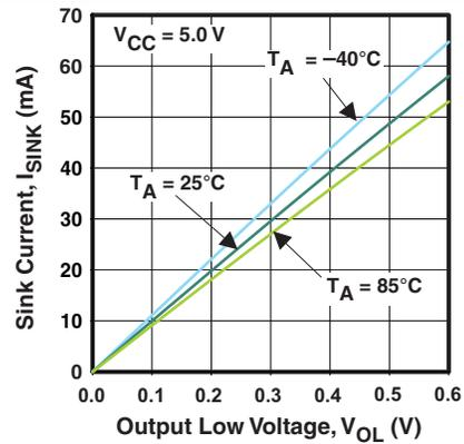
Figure 8. I/O Sink Current vs Output Low Voltage
