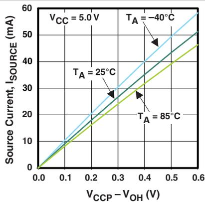
Figure 15. I/O Source Current vs Output High Voltage
