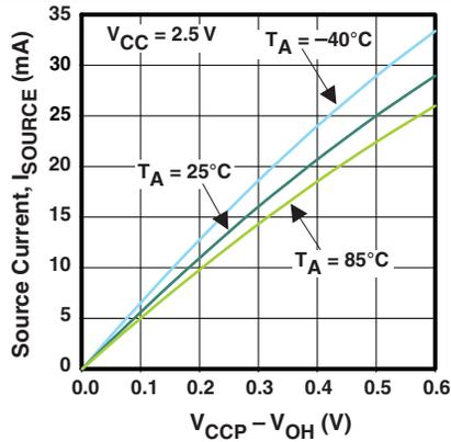
Figure 13. I/O Source Current vs Output High Voltage
