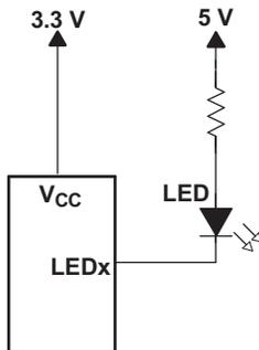
Figure 35. Device Supplied by a Lower Voltage
