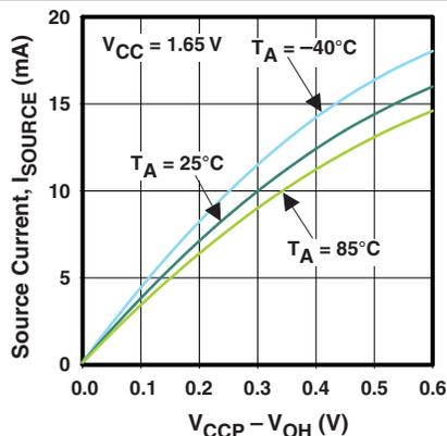
Figure 11. I/O Source Current vs Output High Voltage
