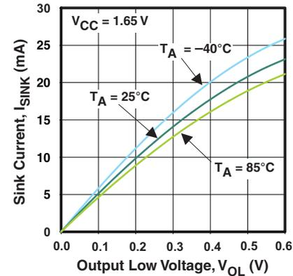
Figure 4. I/O Sink Current vs Output Low Voltage
