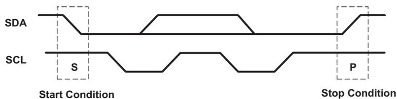
Figure 24. Definition of Start and Stop Conditions
