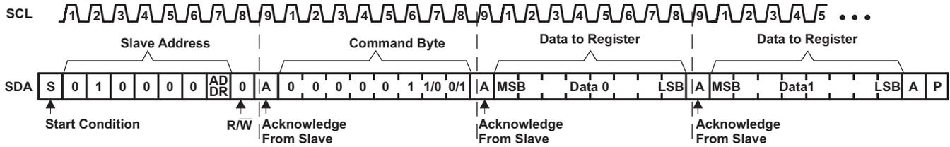
Figure 30. Write to Configuration or Polarity Inversion Registers
