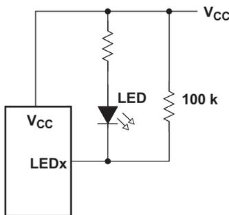
Figure 34. High-Value Resistor in Parallel With LED
