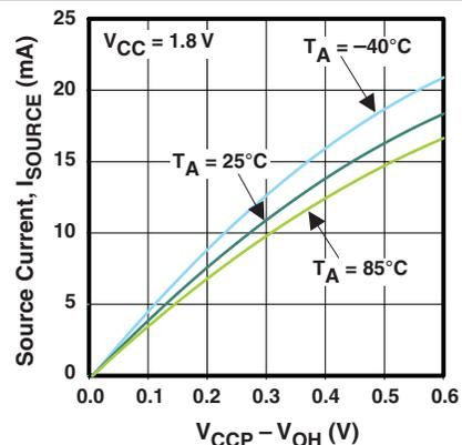
Figure 12. I/O Source Current vs Output High Voltage
