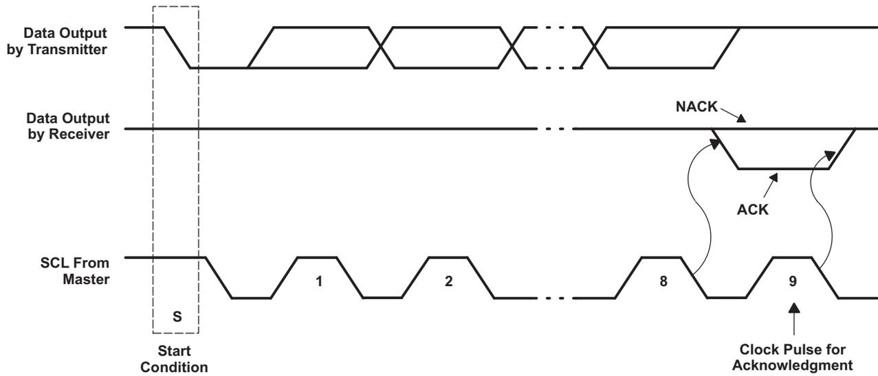
**Figure 26. Acknowledgment on the I<sup>2</sup>C Bus**
