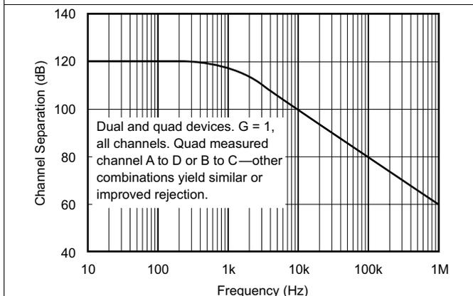
Figure 5. Channel Separation vs Frequency
