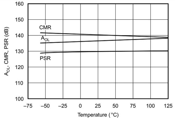
**Figure 10.  $A_{OL}$ , CMR, PSR vs Temperature**
