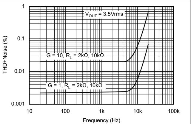
Figure 6. Total Harmonic Distortion + Noise vs Frequency
