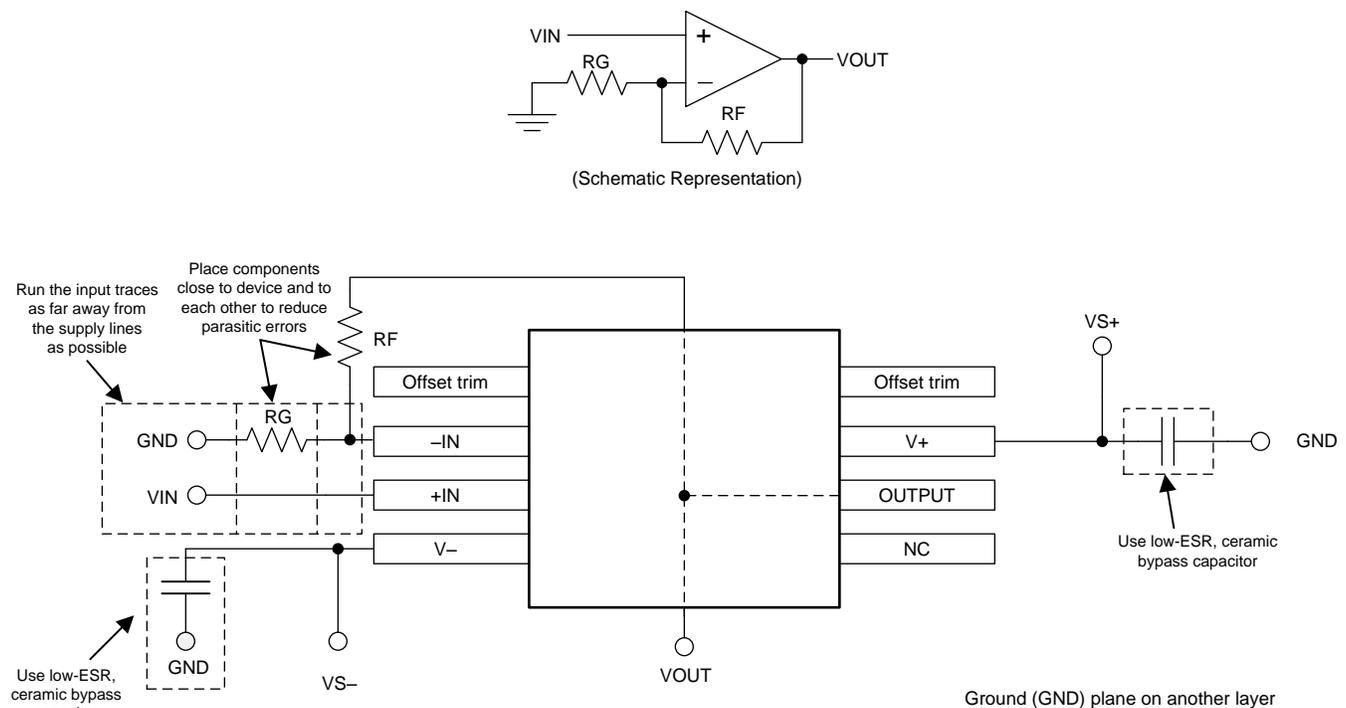
Figure 33. OPA277 Layout Example for the Noninverting Configuration
