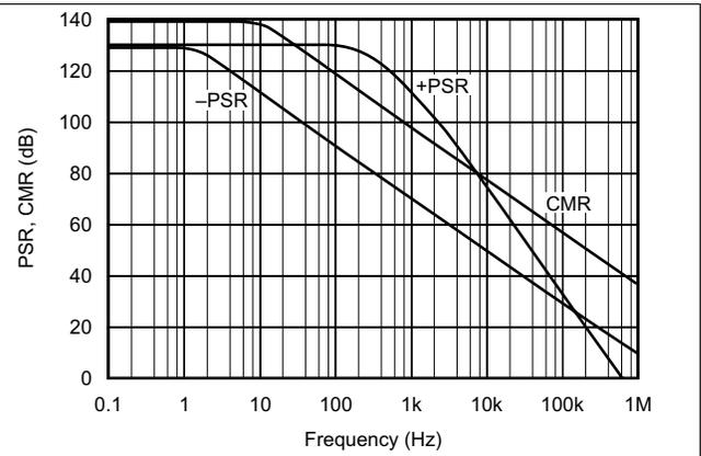
Figure 2. Power Supply and Common-Mode Rejection vs Frequency
