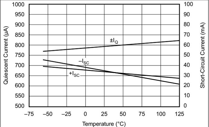
**Figure 12. Quiescent Current and Short-Circuit Current vs Temperature**
