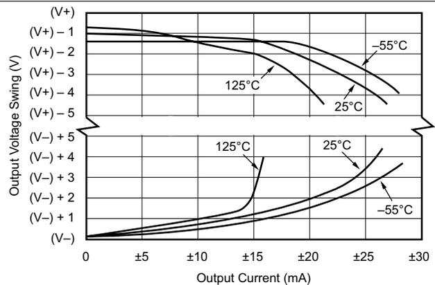
Figure 18. Output Voltage Swing vs Output Current
