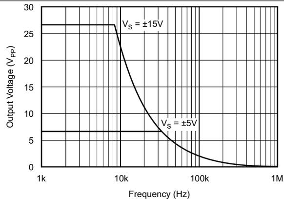
Figure 17. Maximum Output Voltage vs Frequency
