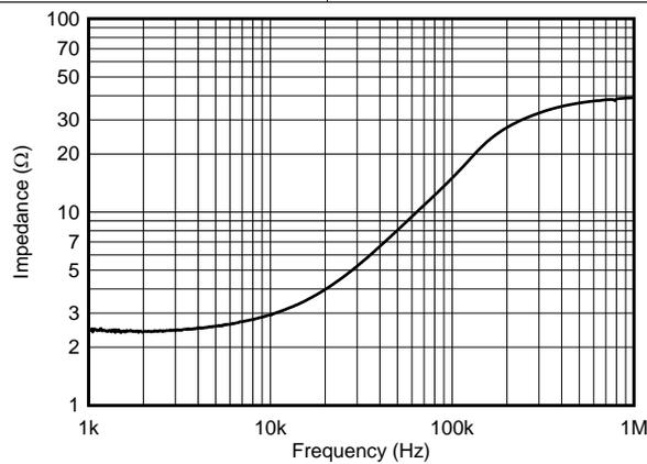
**Figure 23. Open-Loop Output Impedance**
