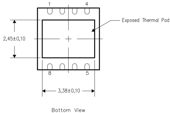
NOTE: All linear dimensions are in millimeters
