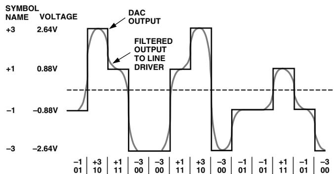
Figure 5. Time Domain Representation of an HDSL Signal
