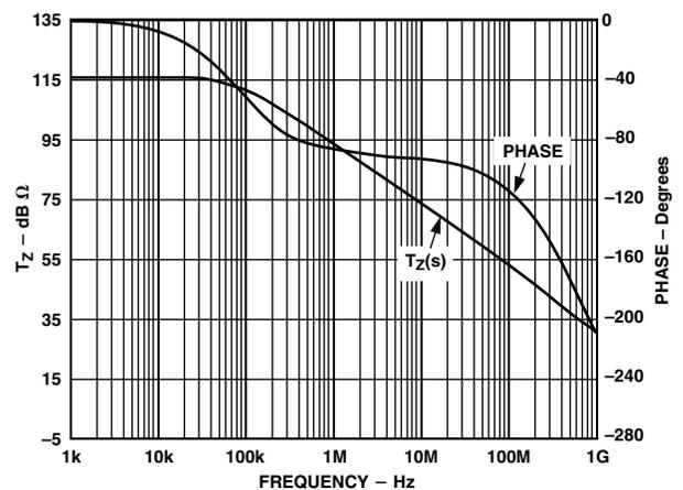
TPC 24. Open-Loop Transimpedance and Phase vs. Frequency
