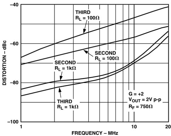
TPC 15. Distortion vs. Frequency;  $V_S = +5 V$
