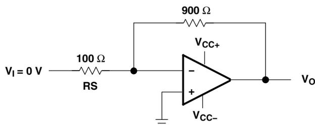
Figure 2. Noise-Test Circuit
