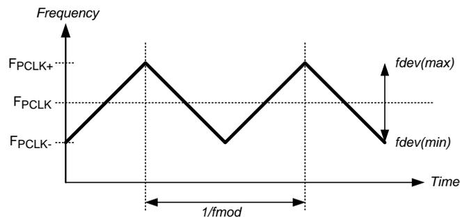
**Figure 26. SSCG Waveform**
