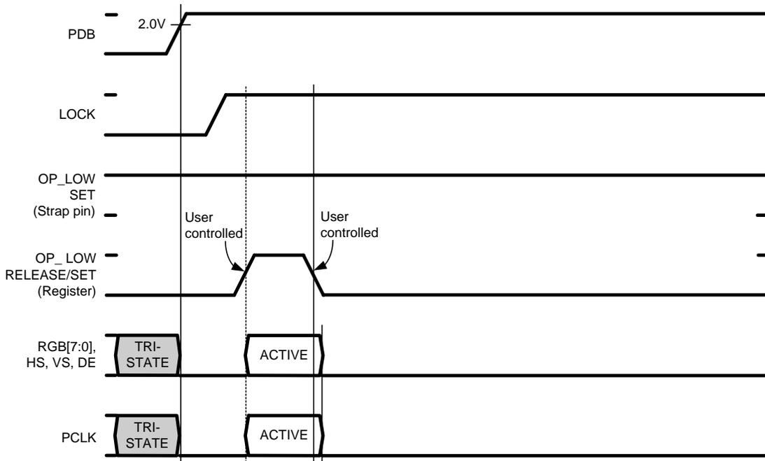
Figure 31. OP\_LOW Manual Set/Reset
