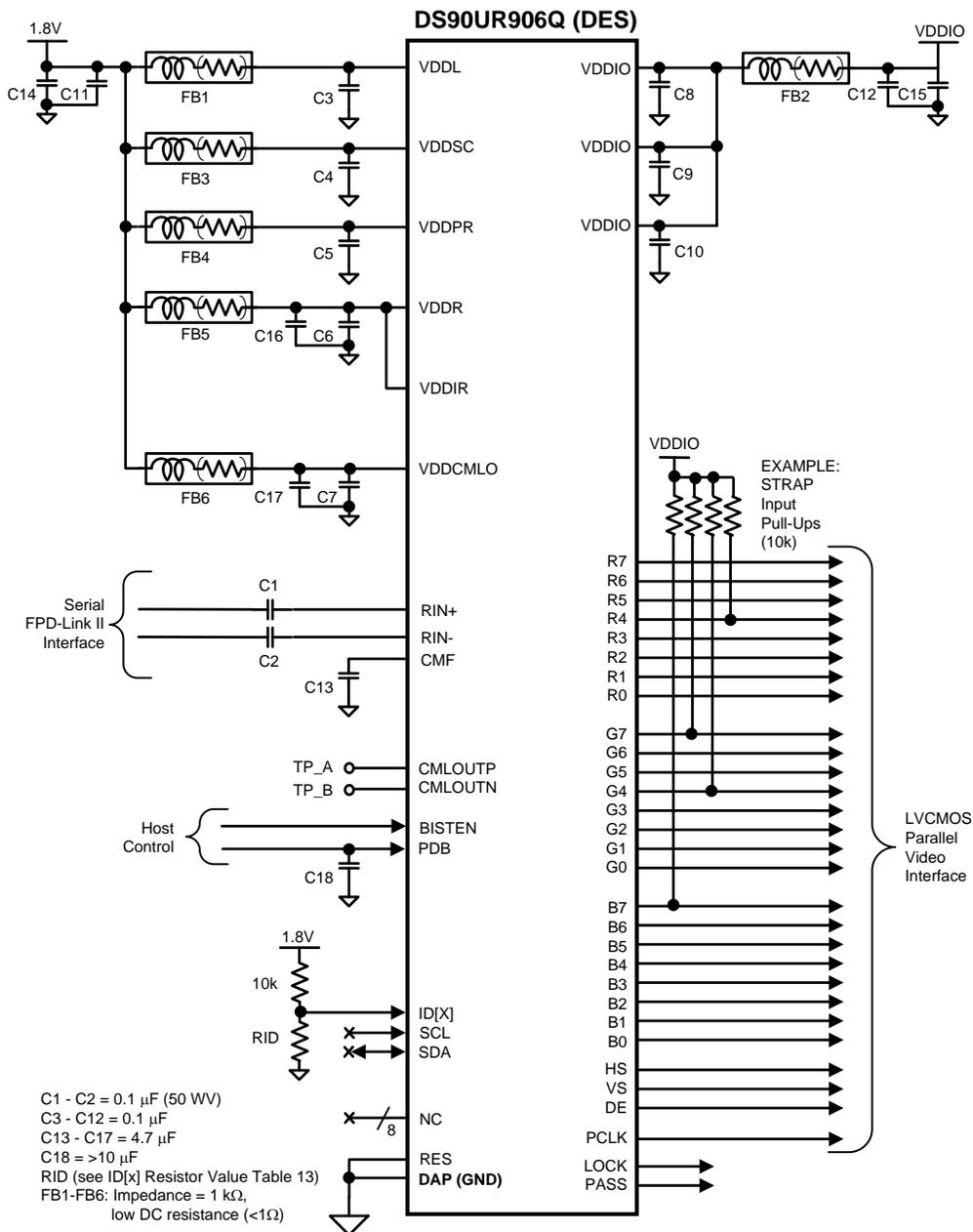
Figure 41. DS90UR906Q-Q1 Typical Connection Diagram — Pin Control
