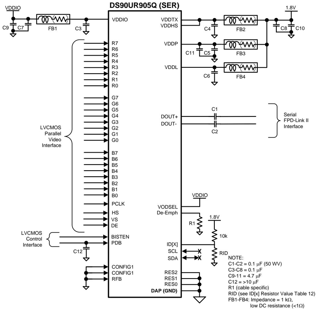
Figure 38. DS90UR905Q-Q1 Typical Connection Diagram – Pin Control
