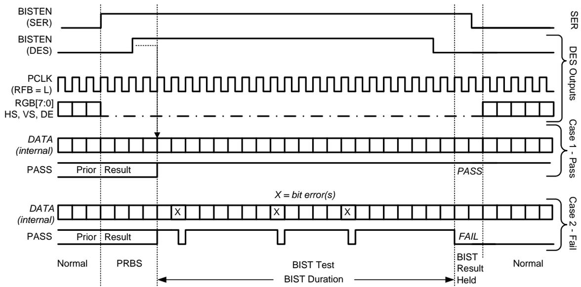
Figure 33. BIST Waveforms
