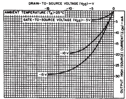
Fig. 8 - Typical output high (source) current characteristics.
