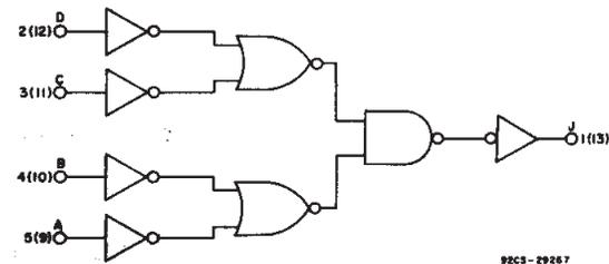
Fig. 9 - Logic diagram for CD4082B (1 of 2 identical gates).
