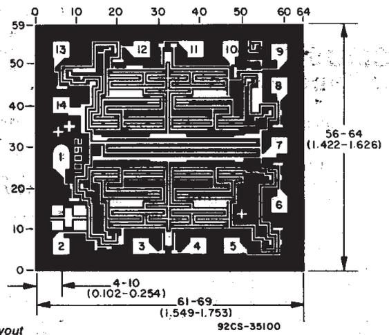
Chip dimensions and pad layout for CD4081B.
