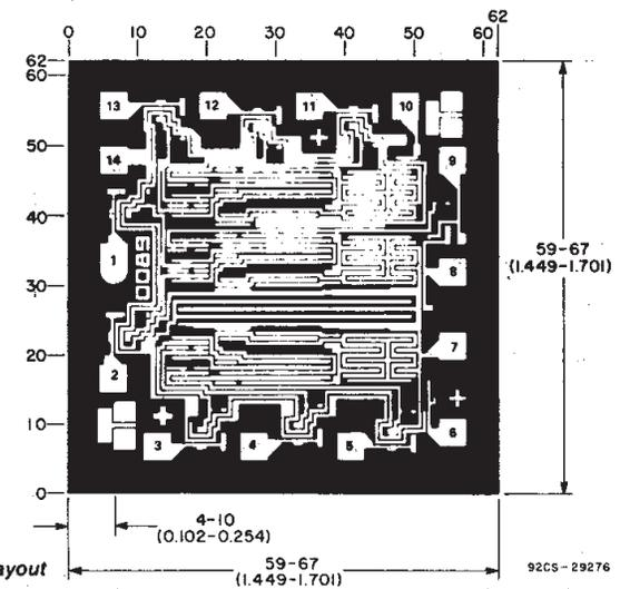
Chip dimensions and pad layout for CD4073B.
