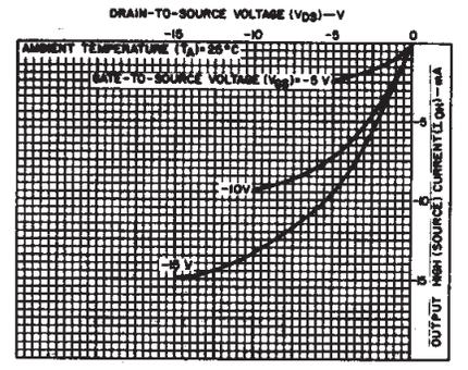
Fig. 10 - Minimum output high (source) current characteristics.
