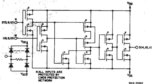
Fig. 1 - Schematic diagram for CD4081B (1 of 4 identical gates).
