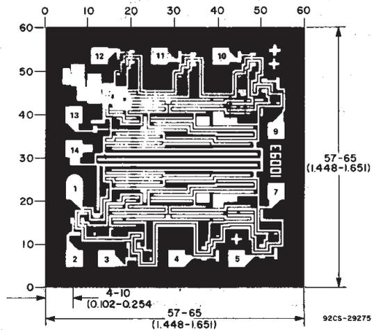
Chip dimensions and pad layout for CD4082B.
