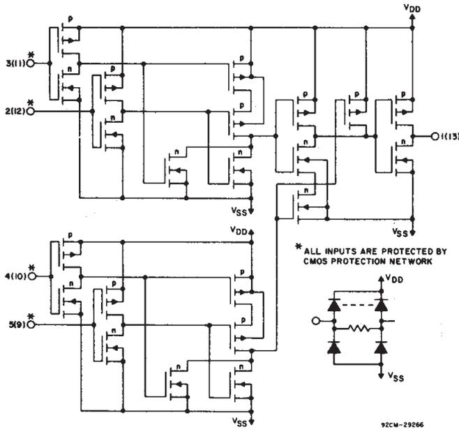
Fig. 7 - Schematic diagram for CD4082B (1 of 2 identical gates).
