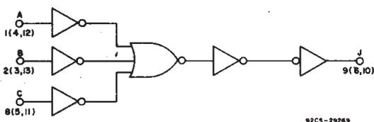
Fig. 13 - Logic diagram for CD4073B (1 of 3 identical gates).
