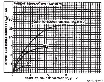
Fig. 5 - Typical output low (sink) current characteristics.
