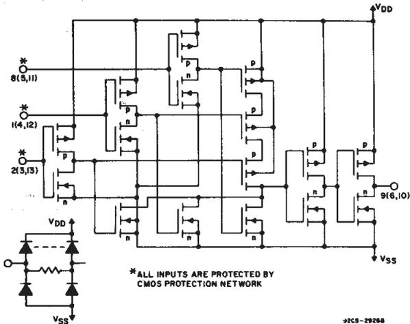
Fig. 11 - Schematic diagram for CD4073B (1 of 3 identical gates).
