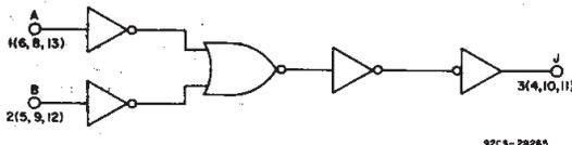
Fig. 2 - Logic diagram for CD4081B (1 of 4 identical gates).
