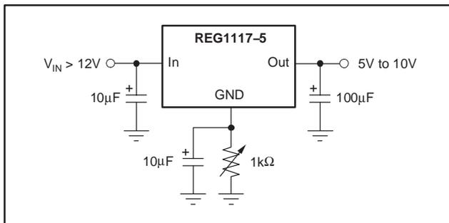
Figure 8. Adjusting Output of Fixed Voltage Models
