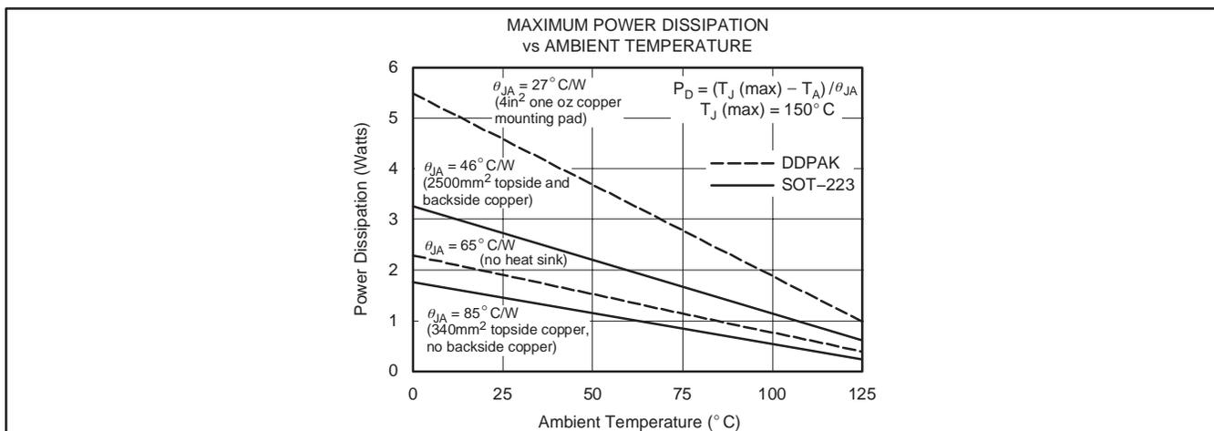
Figure 6. Maximum Power Dissipation versus Ambient Temperature
