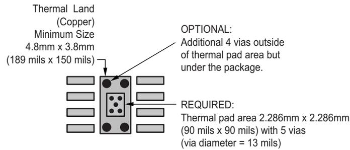
**Figure 41. 8-Pin PowerPAD PCB Etch and Via Pattern**
