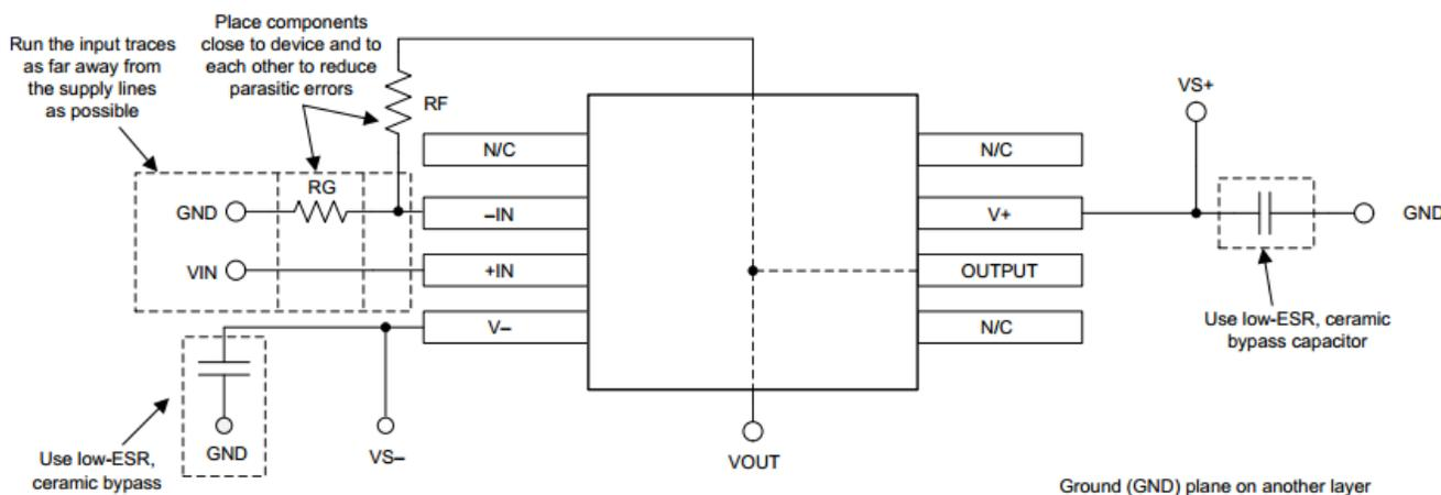
Figure 39. Operational Amplifier Board Layout for Noninverting Configuration
