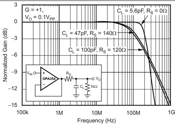
Figure 15. Frequency Response vs Capacitive Load
