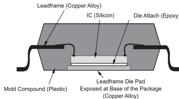
Figure 40. Section View of a PowerPAD Package
