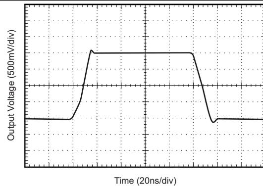
Figure 4. Noninverting Large-Signal Step Response
