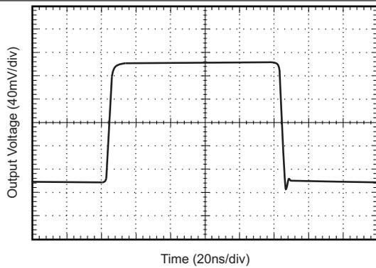
Figure 3. Noninverting Small-Signal Step Response
