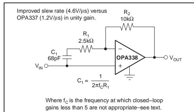
Figure 3. Compensation of the OPA338 for Unity-Gain Buffer
