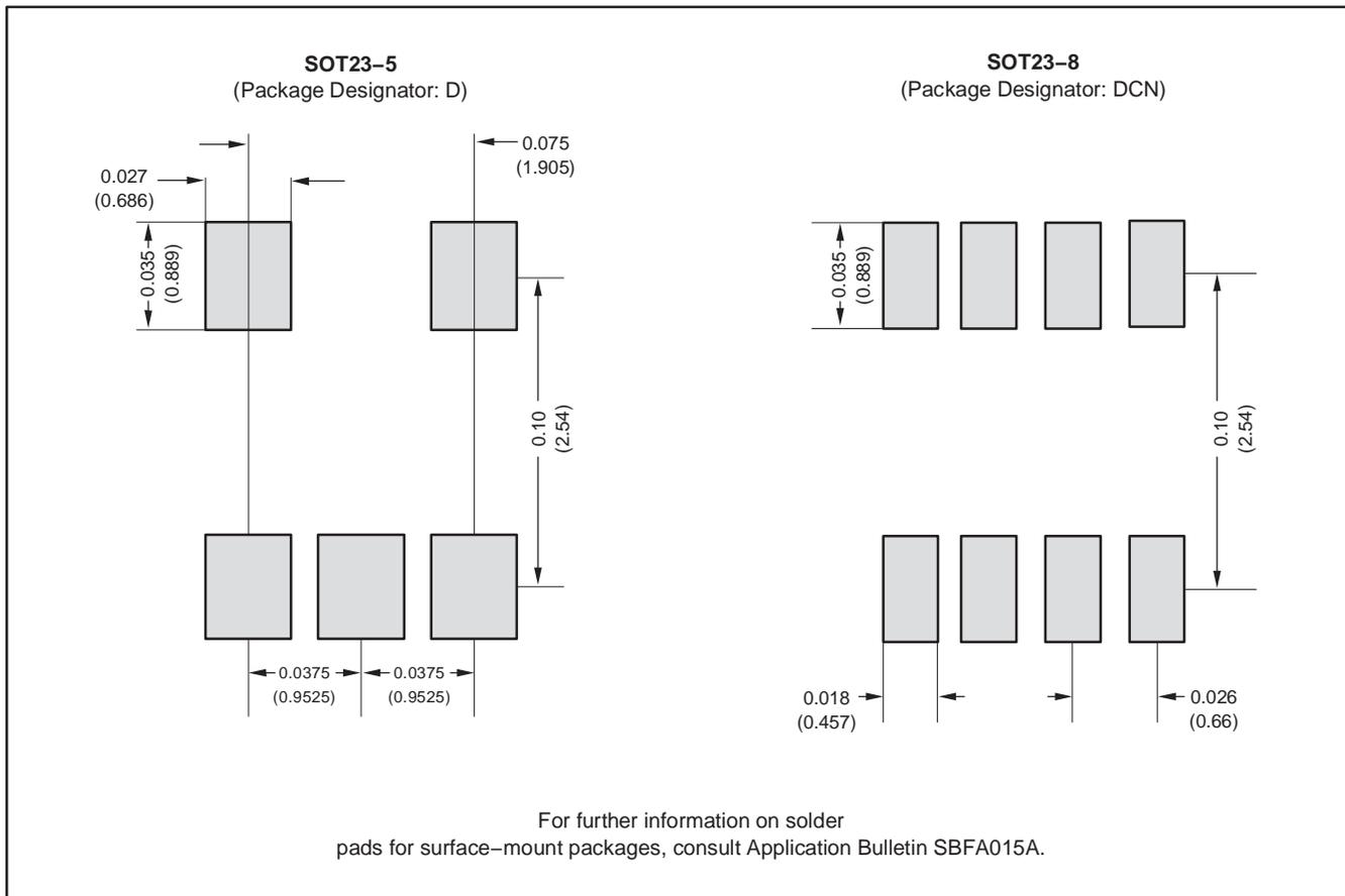
Figure 7. Recommended SOT23-5 and SOT23-8 Solder Footprints
