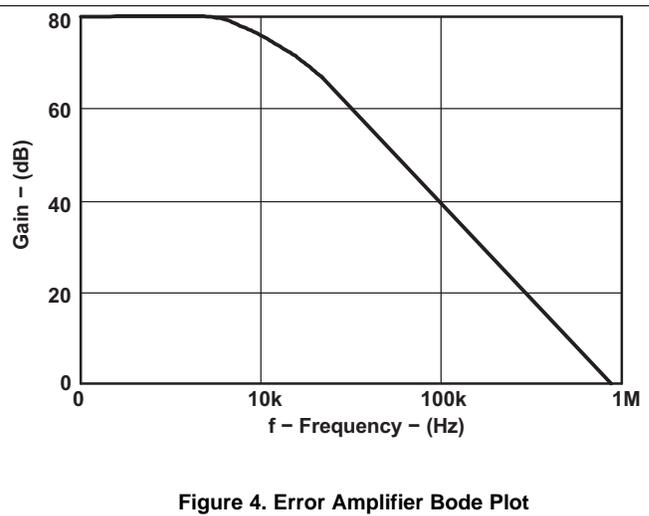
**Figure 4. Error Amplifier Bode Plot**
