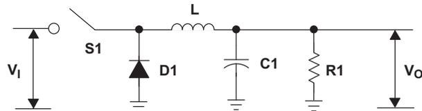
Figure 14. Switching Circuit
