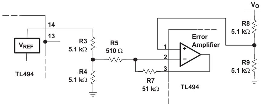
Figure 11. Error-Amplifier Section
