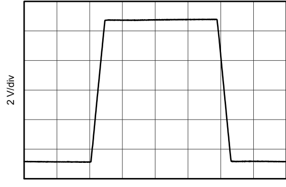
G = -1, R_L = 10 \text{ k}\Omega, C_L = 10 \text{ pF}
