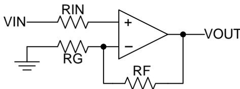
**Figure 16. Operational Amplifier Schematic for Noninverting Configuration**
