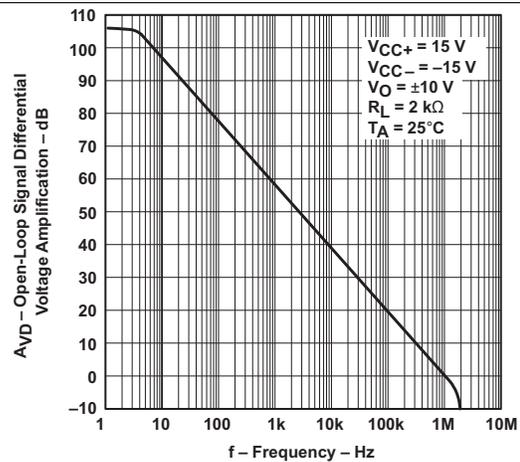
**Figure 7. Open-Loop Large-Signal Differential Voltage Amplification vs Frequency**
