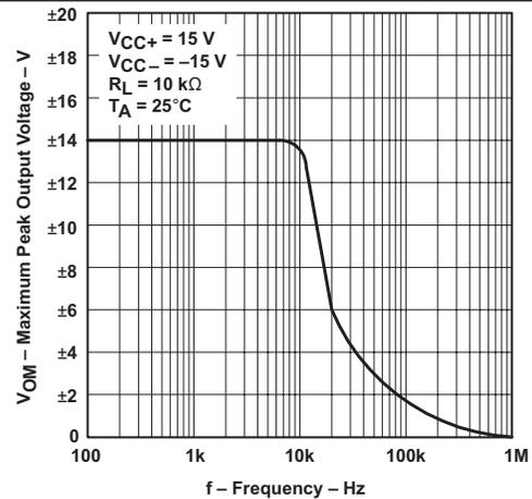
Figure 5. Maximum Peak Output Voltage vs Frequency
