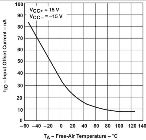
Figure 2. Input Offset Current vs Free-Air Temperature
