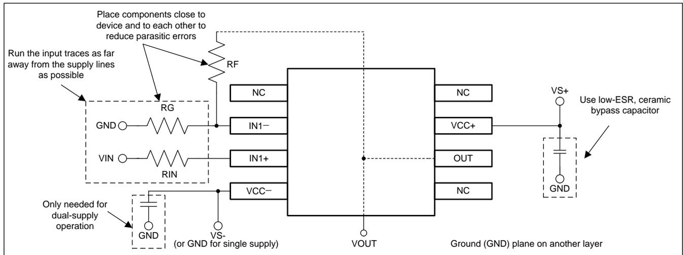
**Figure 17. Operational Amplifier Board Layout for Noninverting Configuration**
