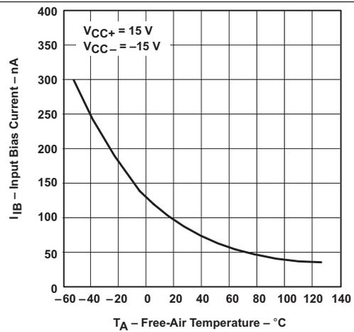
Figure 3. Input Bias Current vs Free-Air Temperature
