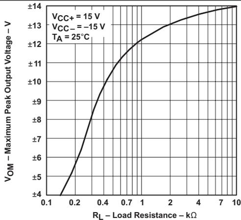
Figure 4. Maximum Output Voltage vs Load Resistance
